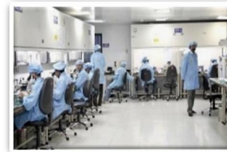
Clean Rooms - Class 10K
