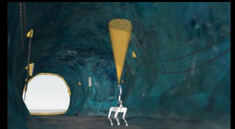
All-terrain, quadruped with manipulators
