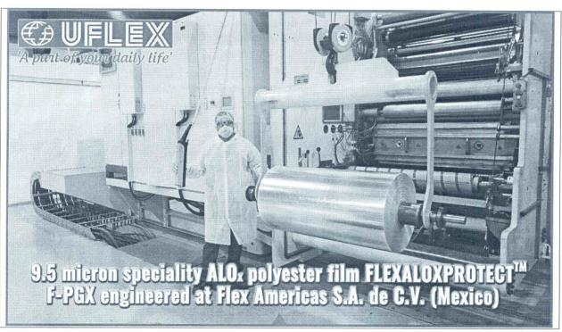
There is a growing demand for transparent flexible packaging that allows retail customers to see-through and check the quality of the product packed inside to their satisfaction. Conventionally metalized films have been used to impart enhanced barrier properties to laminates, but metallization renders the film opaque. The PET ALOx film can offer yet better barrier properties while still being transparent.
