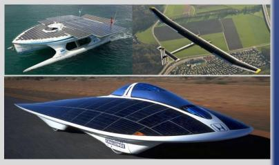
A solar vehicle is an electric vehicle powered completely or significantly by direct solar energy. Usually, photovoltaic (PV) cells contained in solar panels convert the sun's energy directly into electric energy.
