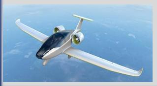
Airbus Group is developing an electric aircraft with Aero Composite Saintonge. The aircraft uses on-board lithium batteries to power the two electric engines.
