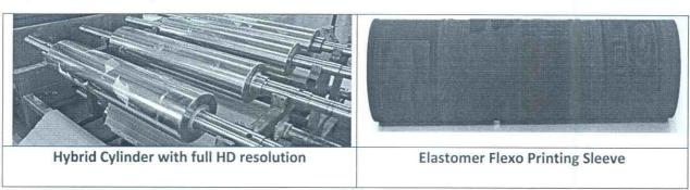
Elastomer flexo sleeves and elastomer flexo plates ensuring exact dot reproduction; no chemical constraint; seamless web printing and reproduction of HD image up to 5080 DPI would be a showstopper.
