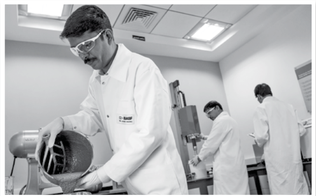
An R&D employee tests concrete additives which are used to change certain physical characteristics of concrete such as flowability. This helps enhance the concrete's performance under various conditions.
