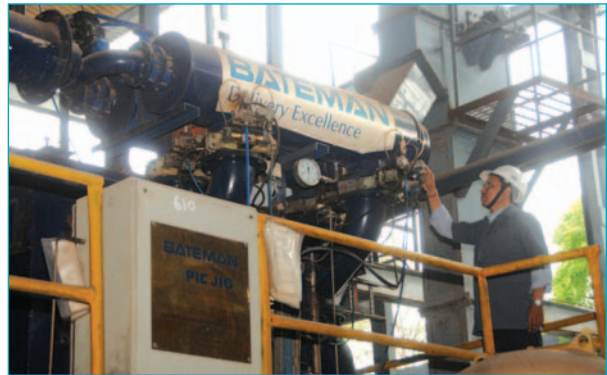
Jig - a gravity preconcentration/ concentration unit at R&D Centre
