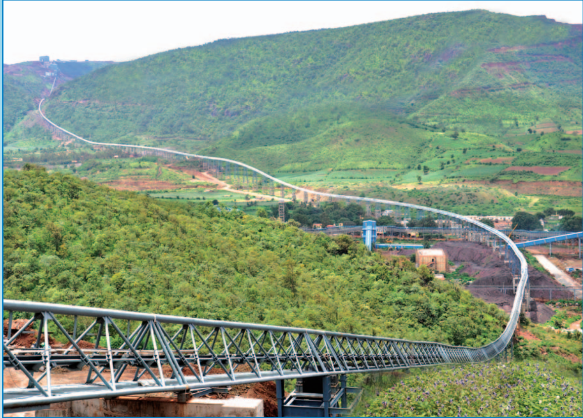
Panoramic view of the 5.2 km long single flight regenerative downhill conveyor belt at Kumaraswamy Iron Ore Mine, Donimalai, Karnataka.
