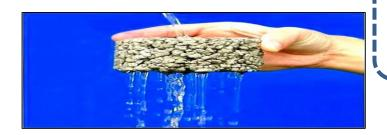
**Perviouscrete**<sup>™</sup> is "Rain water harvesting" concrete.
