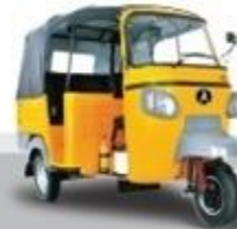
Rear Engine Passenger 3+1 500 kg Payload Capacity
