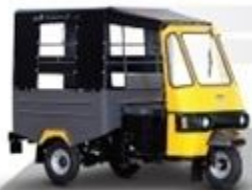
Front Engine Passenger 6+1 500 kg Payload Capacity
