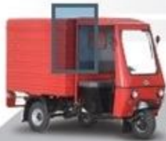
Front Engine Delivery Van 500 kg Payload Capacity
