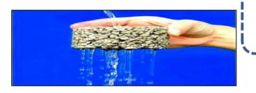
Perviouscrete<sup>™</sup> is "Rain water harvesting" concrete.
