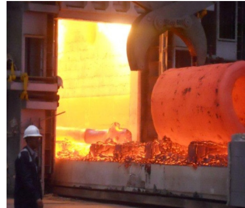
Reheat/ Heat Treatment
