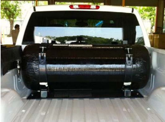
Composite Cylinders mounted on vehicles
