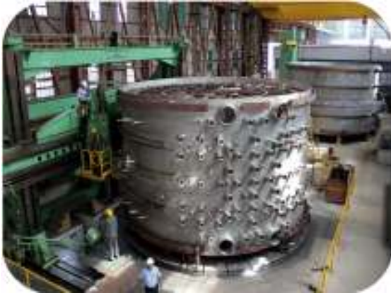
Calandria, 700 MWe Reactor
