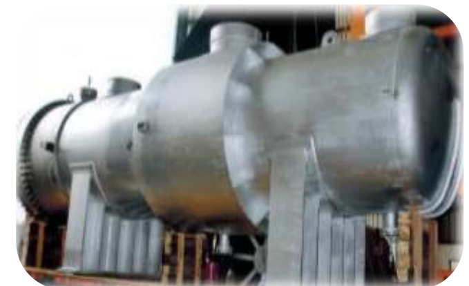
Moderator Heat Exchanger
