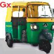
Rear Engine Passenger 3+1 350 kg Payload Capacity
