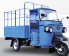
Front Engine High Deck 500 kg Payload Capacity
