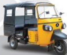
Front Engine Passenger 3+1 500 kg Payload Capacity
