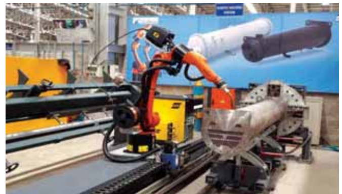
Robotic welding at the manufacturing facility at Wada
