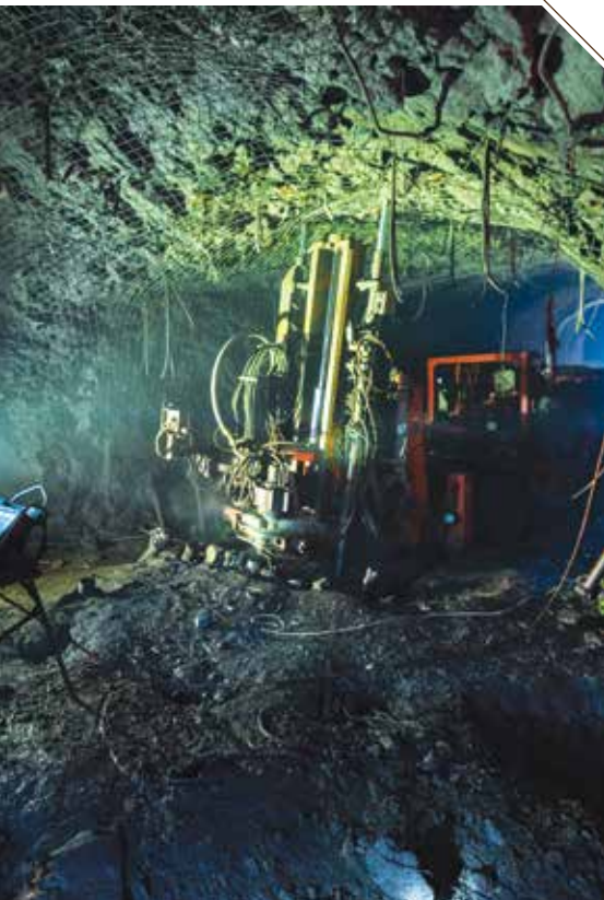
Longhole solo drill rig for accurate drilling
