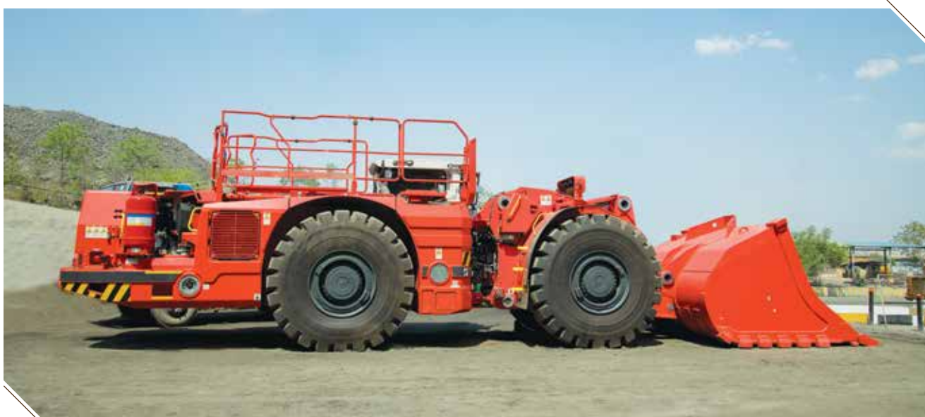
21 MT Load Haul Dump - one of the largest in India
