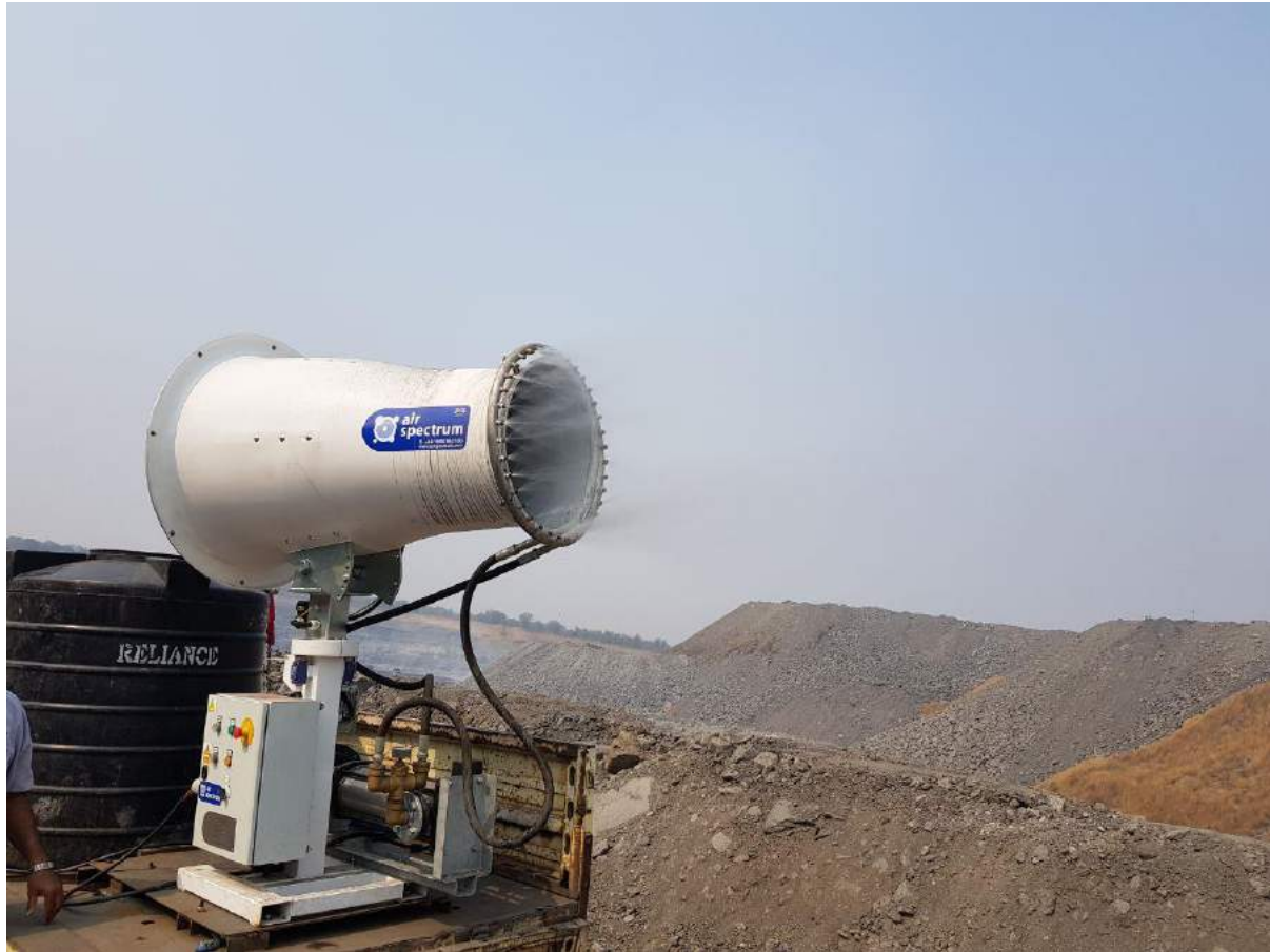
Fig. 30-Dust Controlling Arrangement in CIL Mine
